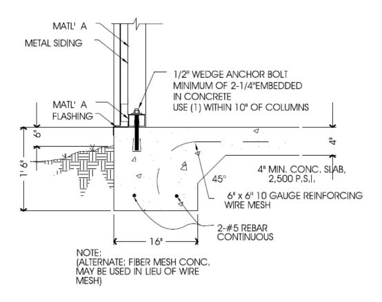
NOTE: FOOTERS MUST BE 16" WIDE X 18" DEEP WITH A MINIMUM OF 4" THICKNESS @ 2,500 P.S.I. CONCRETE. SLAB DIMENSIONS WILL MEASURE 4" WIDER AND 4" LONGER THAN THE STRUCTURE FOOTPRINT TO INCORPORATE THE REVEAL AROUND THE OUTSIDE EDGE.
